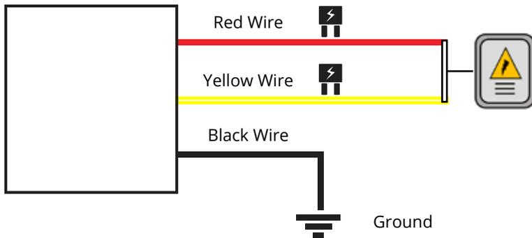
5. **Chassis ground-** Connect to AS11 Black Wire, typically this is a white connection on the trailer harness.
